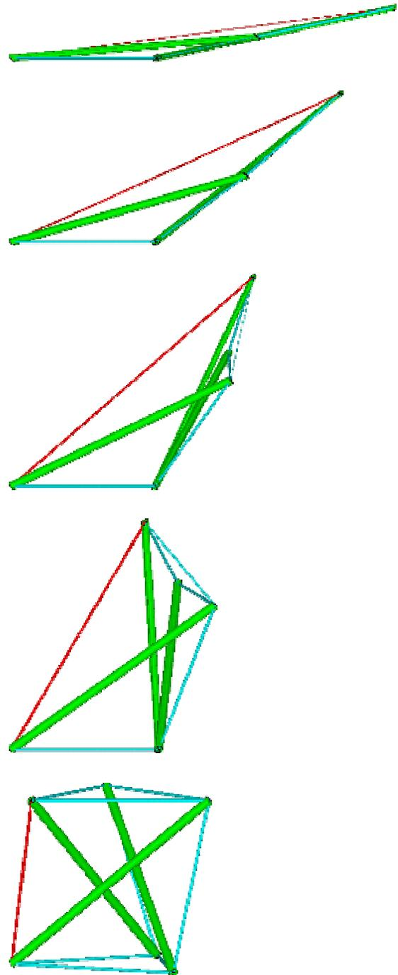
Figure 2. Numerical simulation of the assembling of the tensegrity module.
