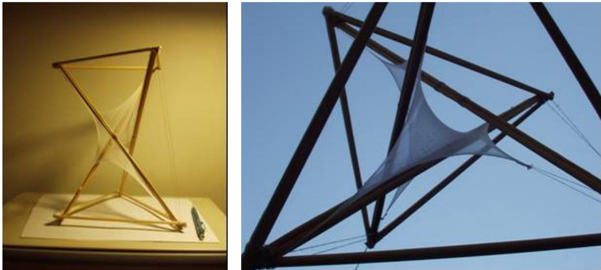
Figure 4. 1:4 scale mock-up of the MFF2, using pantyhose fabric and wood sticks
