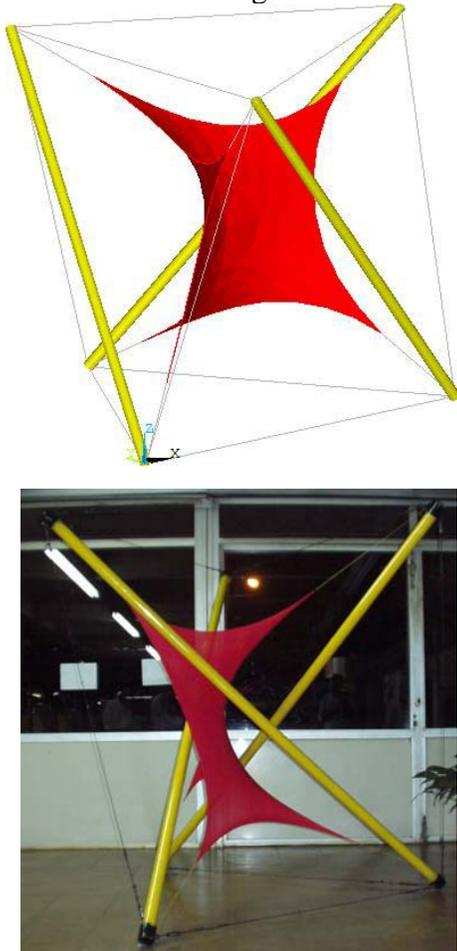
Figure 3. Comparison between the final *Ansys* finite element model, incorporating the tensegrity module, the membrane and the connecting cables, with the real sculpture.
