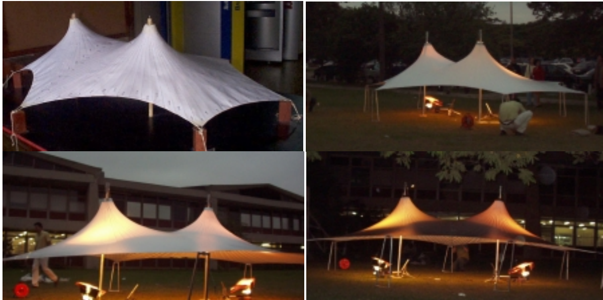
Figure 5: Paper (1:50 scale) and PVC (1:10 scale) models of the double asymmetric conoidal membrane
